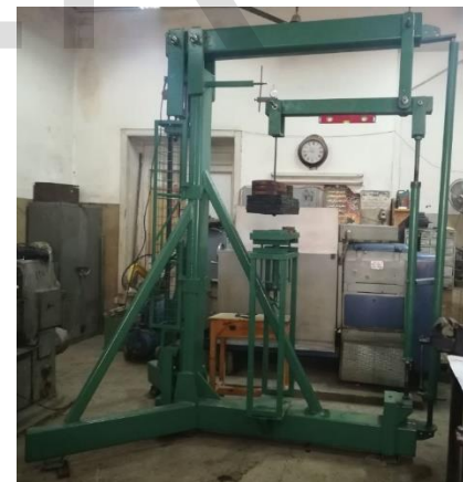
Figure 8: Creep test setup
