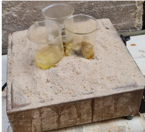
Figure 2: Basalt and Glass FRP tested specimens placed in 70% nitric acid then heated
